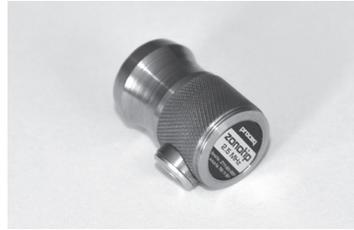
Figura 6: Transductor de 2.5 MHz (S3567)
